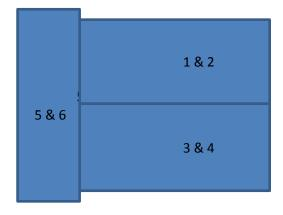
Each module has its own attached legs with bracing and they fold into the overall envelope of the module. The bracing battens are in two halves, hinged and kept rigid by case latches. The outer modules 1 and 4 have two sets of legs at each end and modules 2, 3 and 5 have only one set at one
