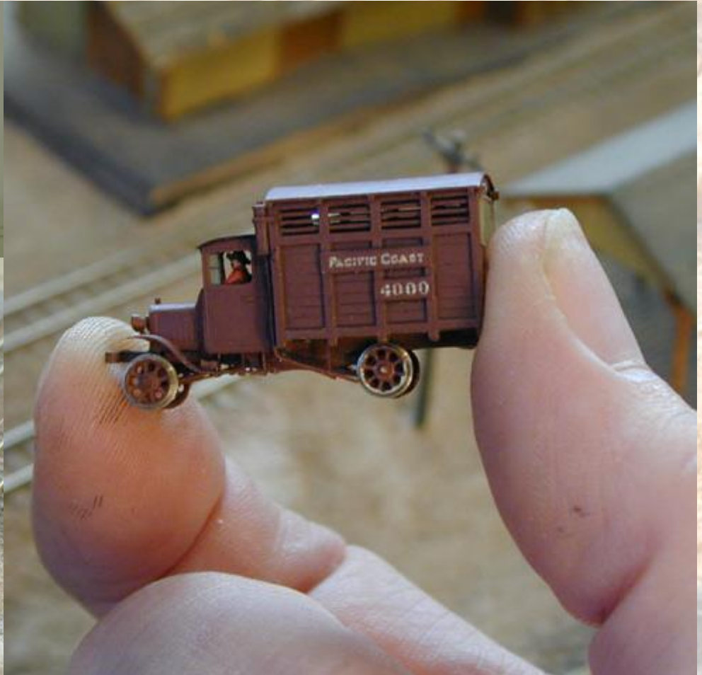
1914 MODEL T FORD RAIL TRUCK SCRATCH-BUILT BY AUTHOR TO RUN ON .256" (6.50 MM) GAUGE TRACK, USING "PAGER" MOTOR
