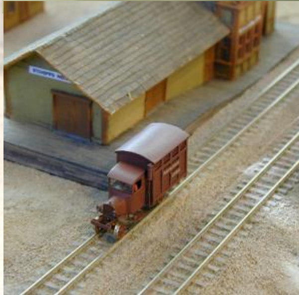
1914 MODEL T FORD RAIL TRUCK SCRATCH-BUILT BY AUTHOR TO RUN ON .256" (6.50 MM) GAUGE TRACK, USING "PAGER" MOTOR
