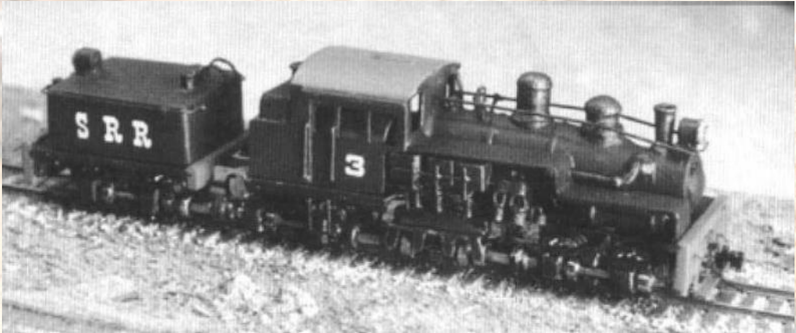
THREE TRUCK SHAY BUILT BY ROGER HORD (AUS) TO RUN ON .256" (6.50 MM) GAUGE TRACK
