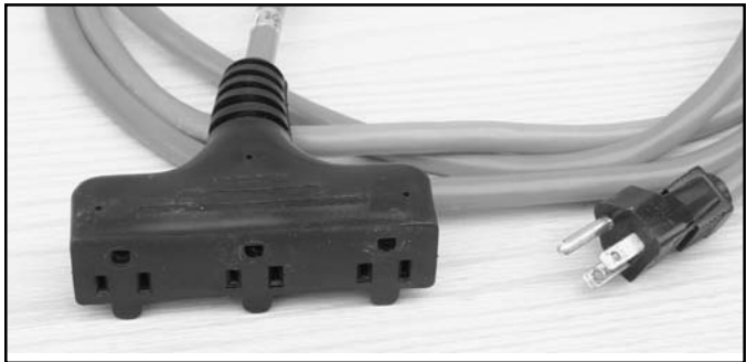
The 25’ extension cord (sometimes called a “Power Block”) came from Ace Hardware and was less than $20. It is rated as “Heavy Duty”, 15 Amp, 14/3 wire in a “SJ” type cord. Over 50’ should be 12/3 Gauge wire. Home built or repaired cords are not accepted.
